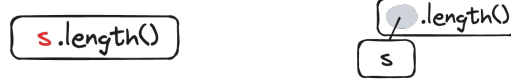
Fig. 2. Example of an incorrect snippet from a student on the left, and its corresponding snippet from the solution on the right from E01. The target of a MethodInvocation is a subexpression and should therefore be represented with a separate node.
